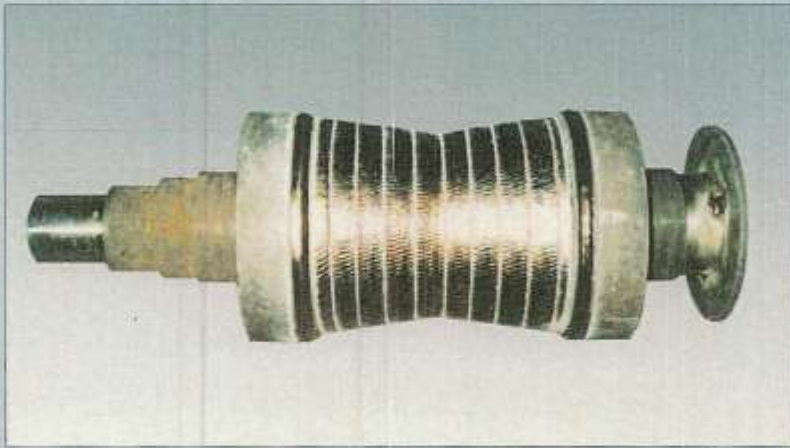
PINCH ROLLER (MHA No.12)
