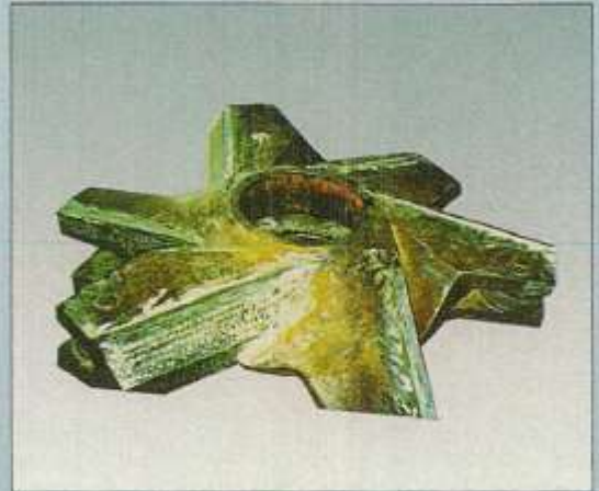
ROTOR FOR REFUSE DISPOSAL (MHA No.12)
