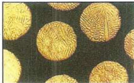
Cross Section Micro Structure of Particle
